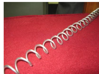
Fig.3: Photograph of the wire coil insert
